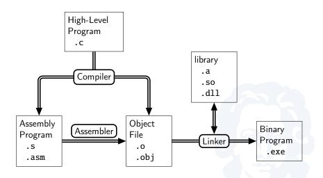
Binary program is machine code, can be passed to
